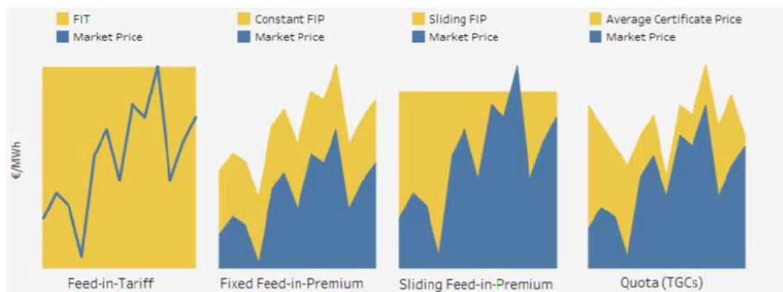
Figure 5-9 Schematic illustration of main RES support schemes and their relation to electricity market price.
