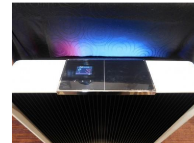
Qarnot's Q.rad Reuses Computing Heat To Provide Warmth To Rooms
